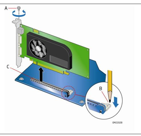
Figure 18. Removing a PCI Express x16 Graphics Card
